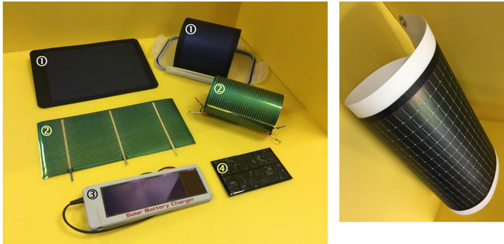
Fig 1. [LEFT] Commercial available solar cells. ① Amorphous silicon thin film, flexible; ② CIGS (Copper Indium Gallium Selenide), flexible; ③ amorphous silicon; and ④ polycrystalline silicon solar cells. [RIGHT] Rollable solar cell
