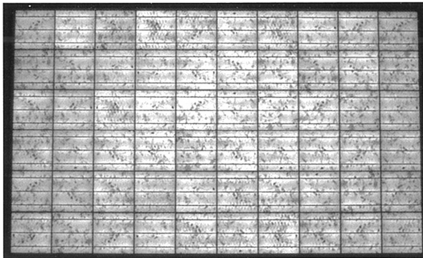
Left: perfect PV module. Right: PV module with micro cracks.
